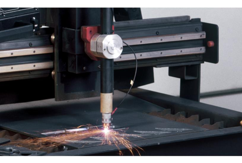
The Sensor PHC is an easy-to-use and reliable voltage-sensing height control for conventional plasma applications.
